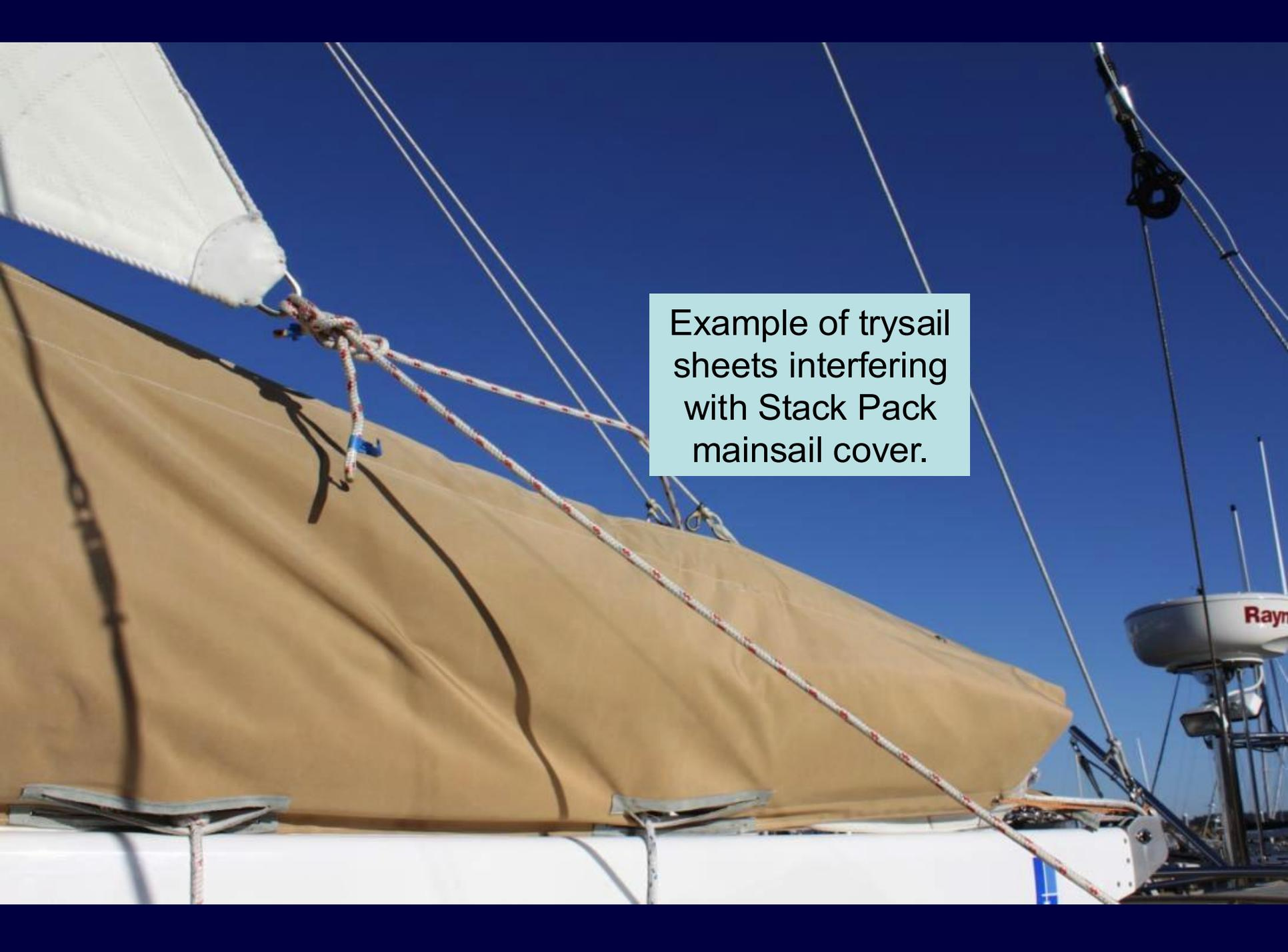
Example of trysail sheets interfering with Stack Pack mainsail cover.
