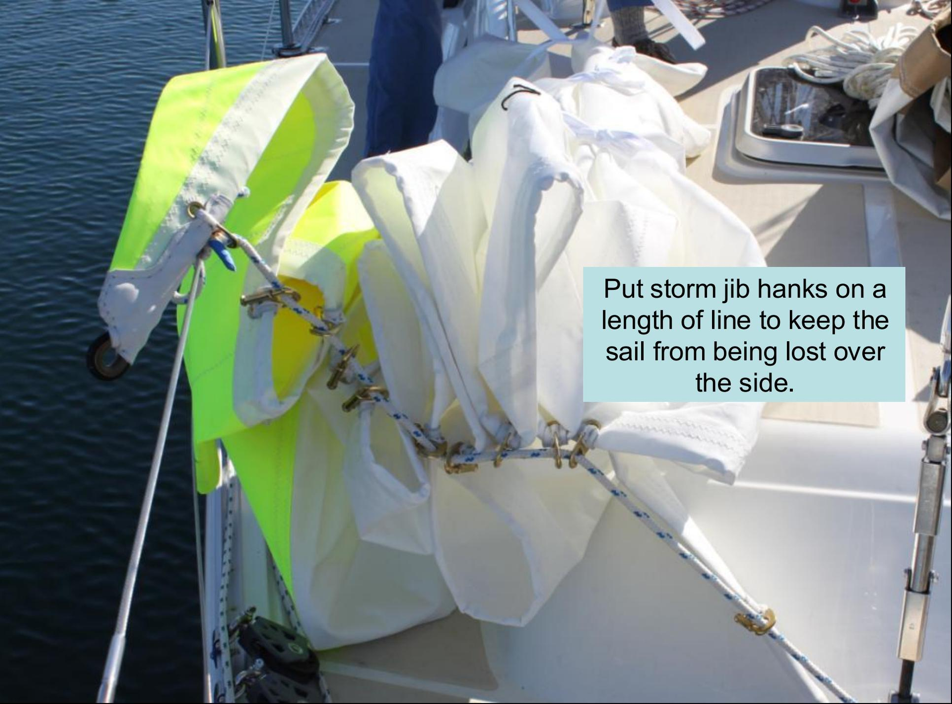
Put storm jib hanks on a length of line to keep the sail from being lost over the side.
