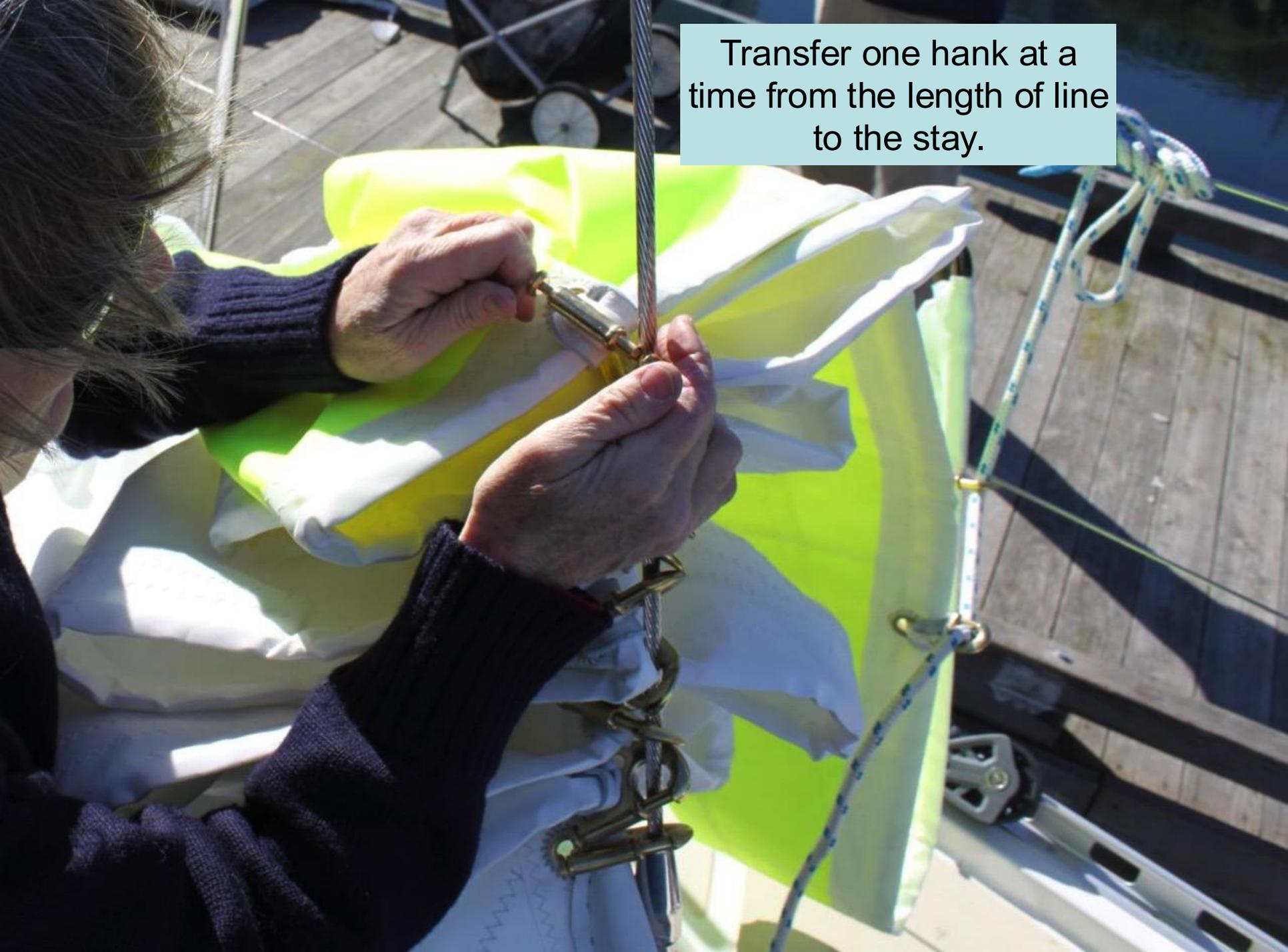
The storm jib is bent on with the bright head panel.
